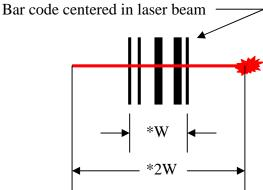
\* Adjust scan distance at minimum 2" (51 mm) or the width of the laser beam is approximately two times the width of the bar code.
