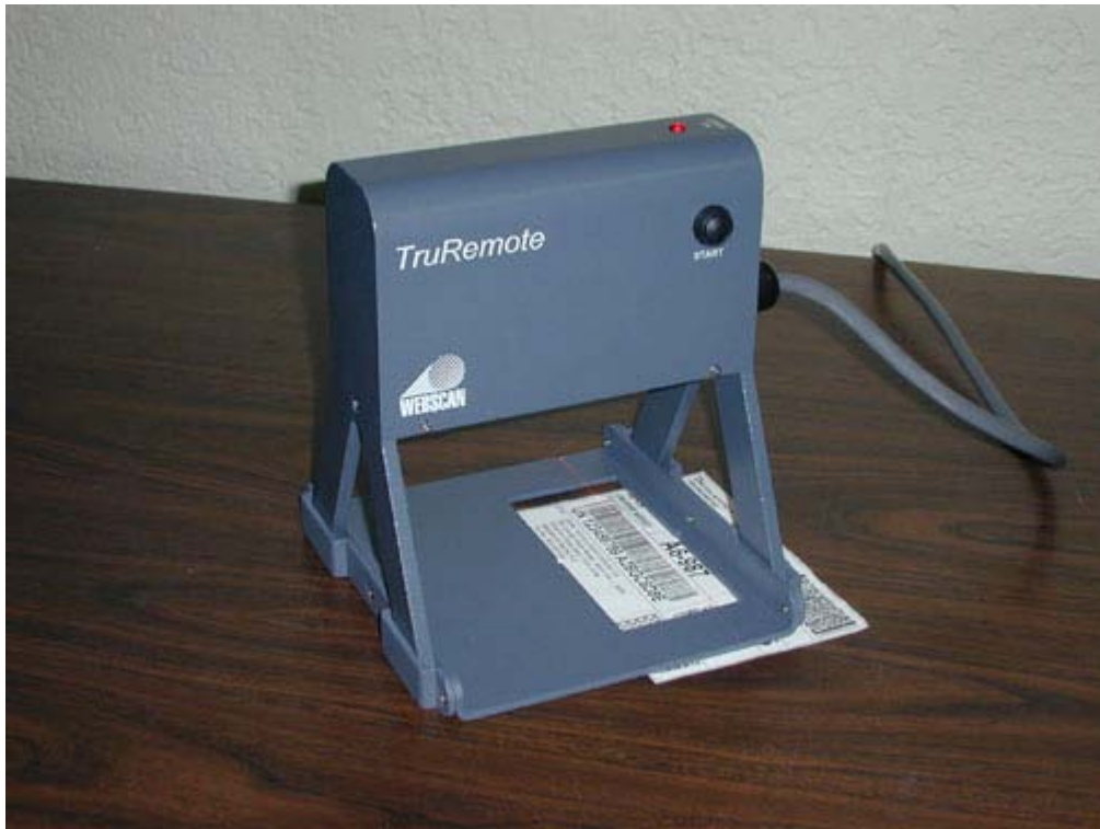
Fig 4.1 – Laser remote placed on top of a symbol, with the symbol to be verified visible through the opening in the guide plate.
